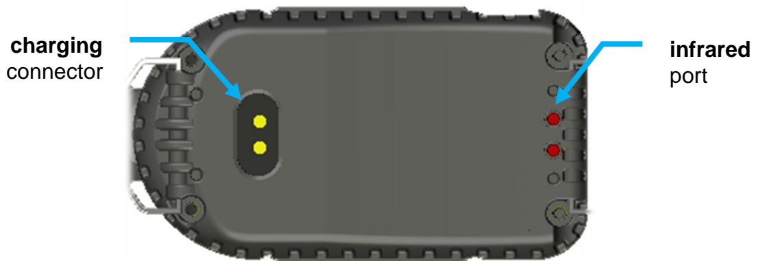
Figure 3-3 SV 104 back view - charging and infrared port (reserved for future use) Figura 3-3 SV 104 vista posterior - carga y puerto infrarrojo (reservado para uso futuro)
