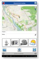
SvanMobile is an application for Android devices that uses the Bluetooth connection to control the SVAN977. It allows the user to trigger measurements, edit settings, rename files and view the results remotely.
