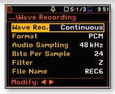
Time signal recording means recording the raw signal samples with defined frequency up to 48 kHz. Analysis of the raw signal is used whenever frequency analysis is not sufficient. Post-processing of wave files such as calculation of tonality is available in SvanPC++ program.
