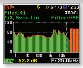
With a special microphone and 1/3 octave or FFT analysis SVAN977 provides analysis of the ultrasounds up to 40 kHz. The ultrasound band is normally considered as the frequency range above 20 kHz. Ultrasound is used in a number of industrial processes such as cleaning, drilling or welding. It is also used in hospitals for medical procedures.
