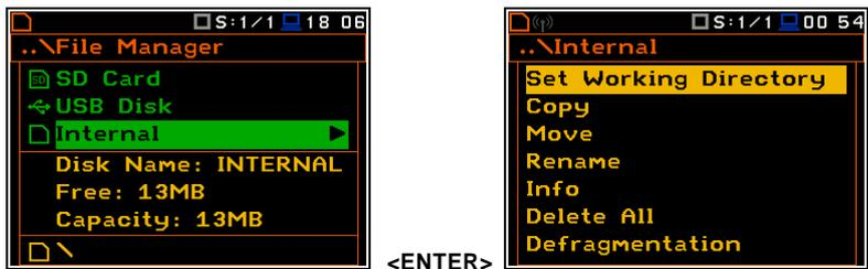
List of operations for the Internal instrument memory
