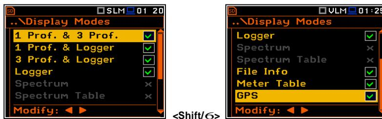
**Display Modes window in the Sound Level Meter mode**
