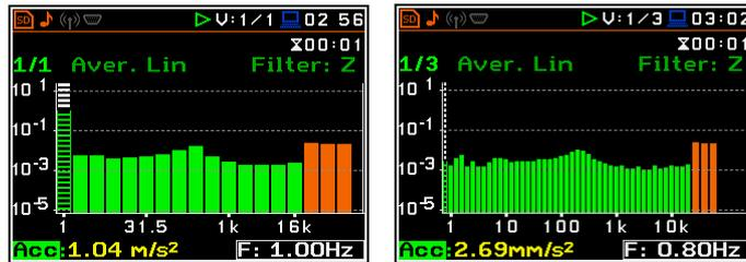
**Displays in Spectrum view for 1/1 Octave and 1/3 Octave function (Vibration modes)**
