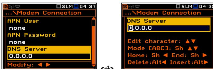
**Modem Connection window; DNS Server address entering**
