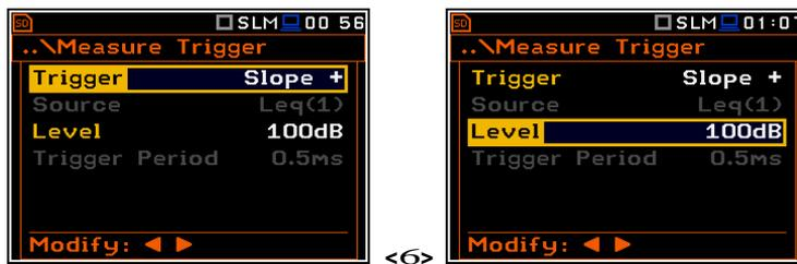
**Measure Trigger windows with not active Source signal line**
