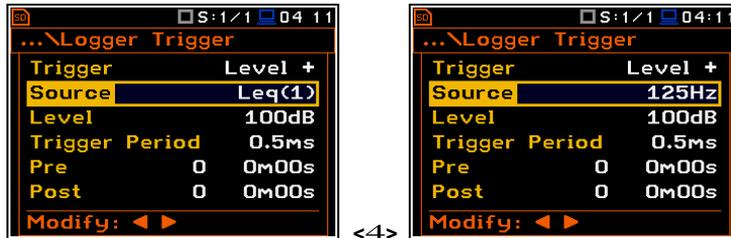
Logger Trigger windows with the active Source signal line (1/1 Octave mode)
