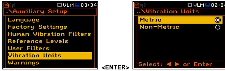
**Auxiliary Setup list, the Vibration Units window opening**
