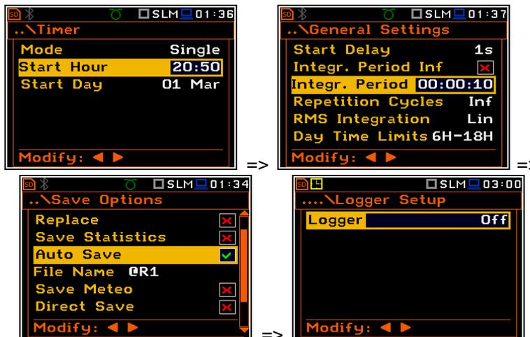
**Exemplary settings made for the desired execution of the Timer function**
