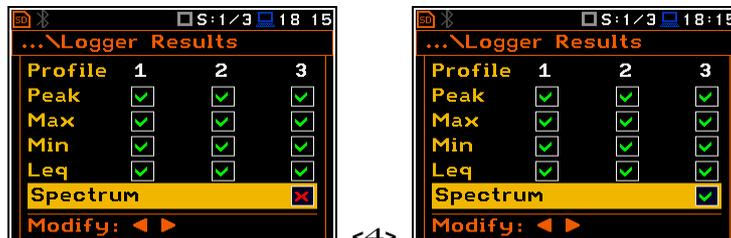
**Spectrum windows with disabled and enabled savings of 1/1 Octave spectrum**
