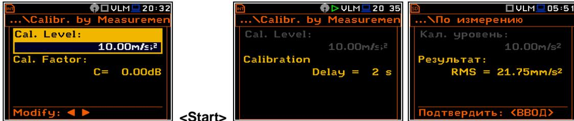
Displays during the calibration measurement
