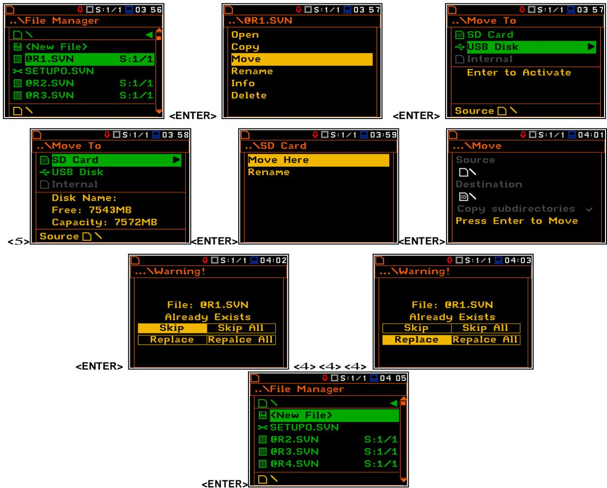
**Moving the file from the Internal memory to SD Card**
