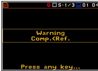
**Display with warning that compared results are lower than reference results**
