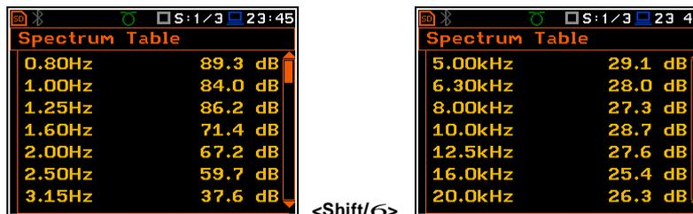
**Displays in Spectrum Table view for 1/3 Octave function (Sound modes)**
