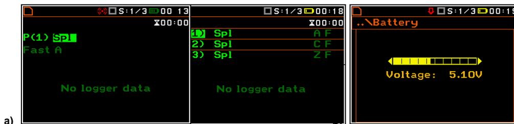
**Displays with the “Battery” icon (a) and in the Battery window (b)**
