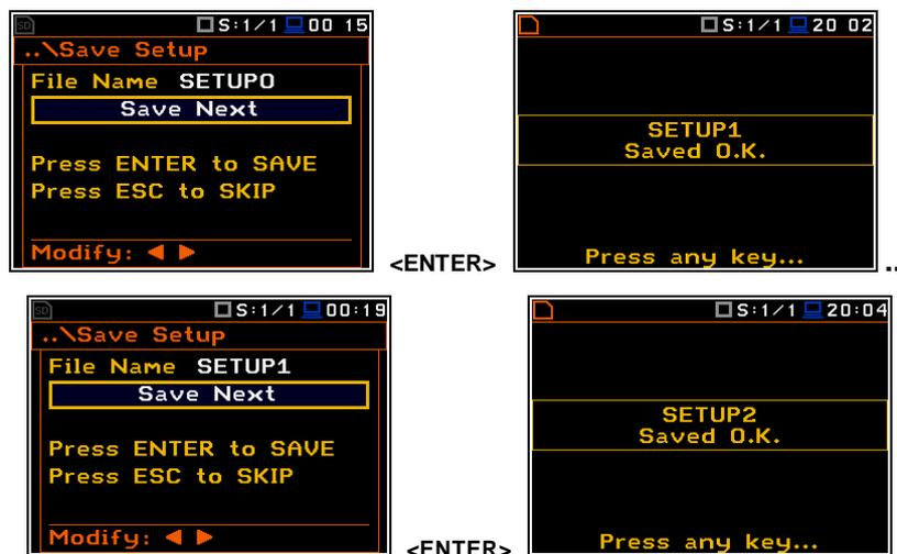
**Displays in the simplified edition of the Setup file name and saving operation execution**
