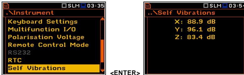
Instrument list; the Self Vibration window opening
