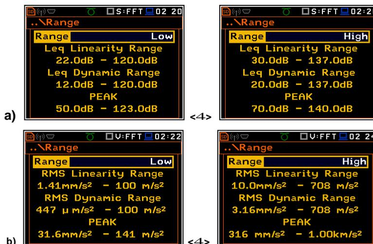
**Range window in FFT analyser in Sound a) and Vibration b) modes**
