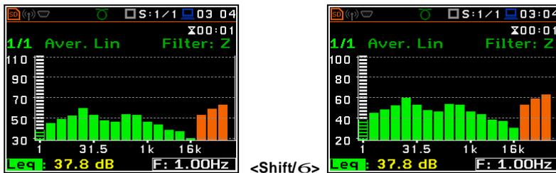
**1/1 Octave analysis with the shifted horizontal axis in relation to vertical one**
