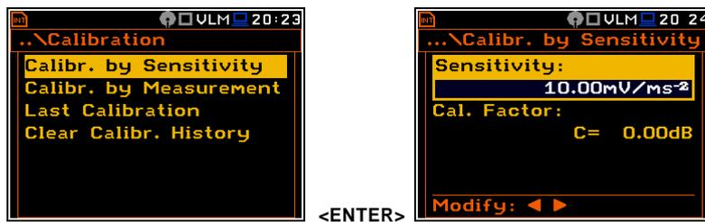
Displays with the selected calibration mode and after entering this mode
