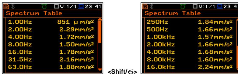
**Displays in Spectrum Table view for 1/1 Octave function (Vibration modes)**
