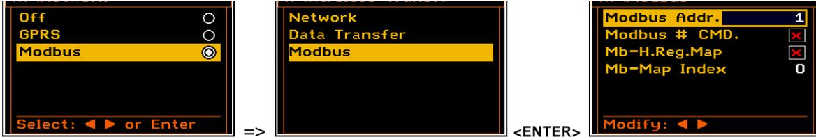
**Wireless Transfer window when Modbus option is chosen**
