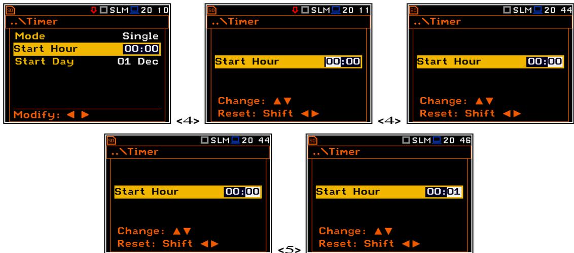
**Timer windows; setting hour and minute for the instrument’s switching on**
