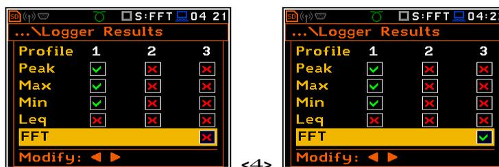
**FFT windows with disabled and enabled savings of FFT spectrum**
