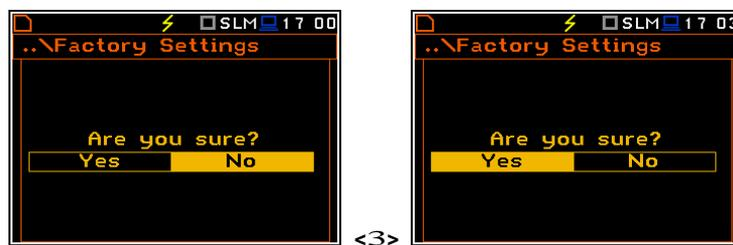
**Displays with the request for the confirmation for the Factory Settings execution**
