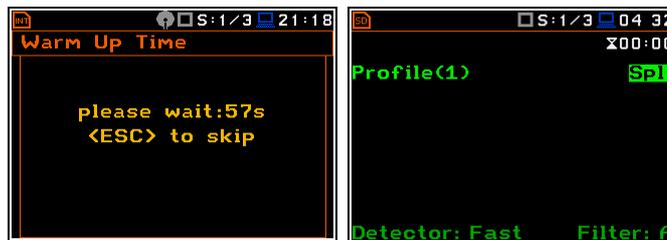
**Displays after switching on the instrument in Sound mode**
