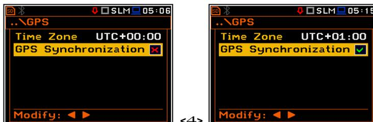
IEPE Current windows; the GPS Synchronization switching on
