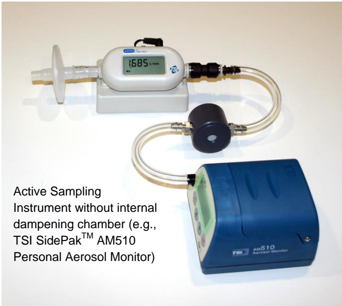
Figure 2-3 Typical Dampening Module Set Up
