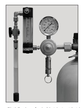
off both "break away" ends of the tube, insert the tube into the tube holder with the directional arrow pointing down, and adjust the flowmeter to the specified flow rate. Allow the prescribed flow time to pass. A precisely measured volume of air is injected into the tube where it contacts the reagent.
