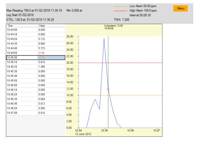
The top area displays the general details of the log and of how the Cub was configured at the time.
