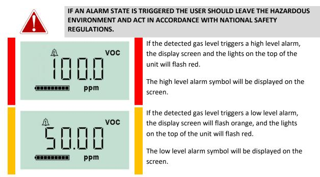
Depending on how the Cub was set up, an alarm may also sound and the unit may vibrate.
