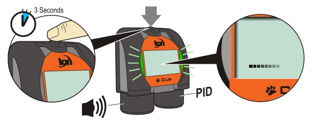
Finally, a short alarm will sound, and the LEDs will flash green. The main gas detection display screen (see below) will then be displayed. Your Cub is now ready to use.
