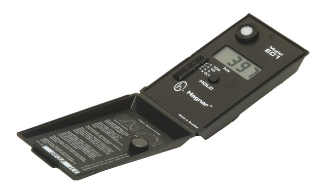
The Hagner Digital Luxmeter is a small, handy and extremely easy-to-use instrument for accurate measurement of illuminance over a range of 0.1-200,000 lux. With both automatic zeroing and on/off switch, the only controls needed are a four-position range selection switch and a hold button for retaining the display value.
