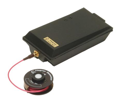
The Hagner Digital Luxmeter is a small, handy and extremely easy-to-use instrument for accurate measurement of illuminance over a range of 0.1-200,000 lux. With both automatic zeroing and on/off switch, the only controls needed are a four-position range selection switch and a hold button for retaining the display value.
