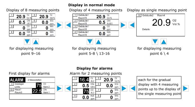
The display is backlit; the light intensity can be increased using any control button. In the event of a gas alarm or faults, the display lighting is automatically activated with a red background.
