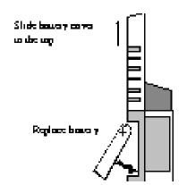
For battery replacement slide the battery cover up. Then take the old battery out and replace it with a new one.
