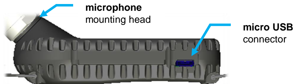
Figure 3-2 SV 104A side view – microphone and micro USB connector
