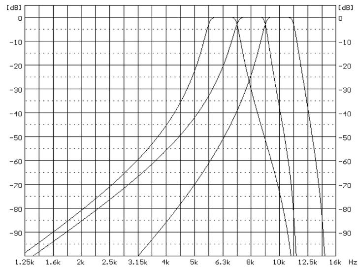
**1/3 octave filters for 8.0 kHz 1/1 octave filter**
