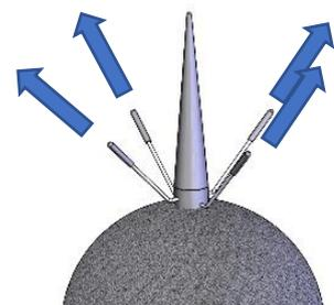
1. Screw the assembled instrument on the M14 thread of the mast rotating it clockwise.
