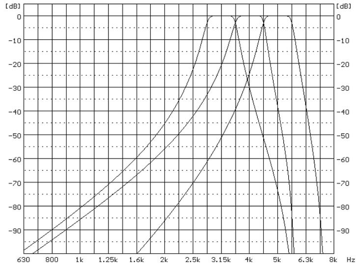
**1/3 octave filters for 4.0 kHz 1/1 octave filter**
