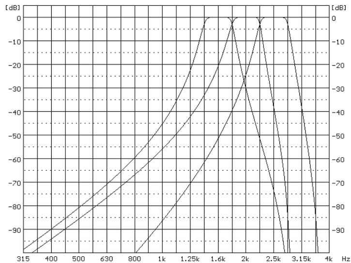
**1/3 octave filters for 2.0 kHz 1/1 octave filter**
