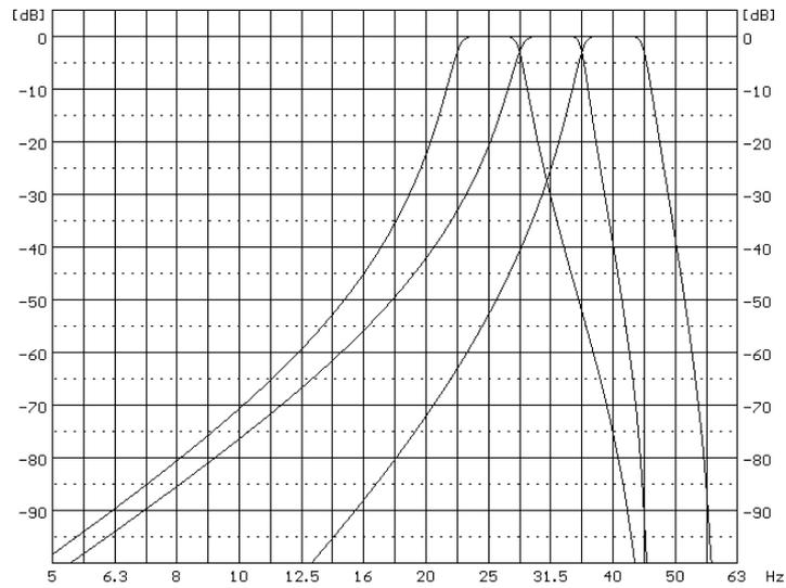
**1/3 octave filters for 31.5 Hz 1/1 octave filter**
