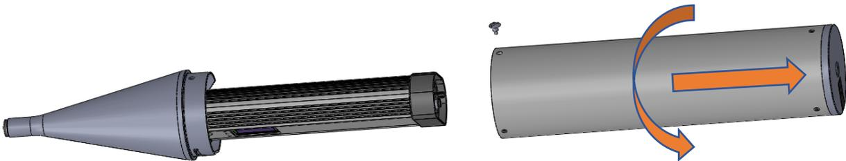
3. Unscrew four bolts and detach the bottom plastic cover of SV 307 to have access to the SIM card and micro SD-card slots.
