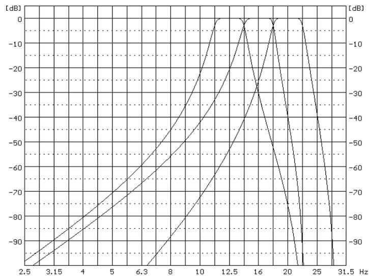
**1/3 octave filters for 16.0 Hz 1/1 octave filter**
