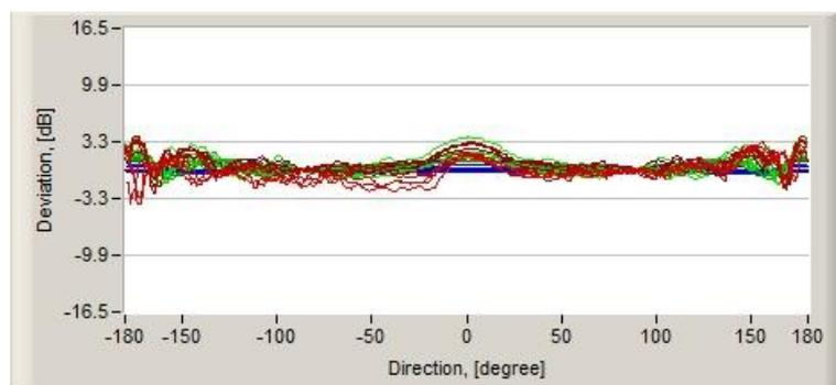
Below the directional characteristics and tolerances for 90 degree and 0 degree incidental angles are presented.
