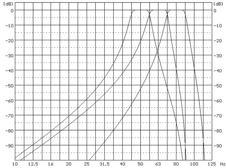
**1/3 octave filters for 63.0 Hz 1/1 octave filter**
