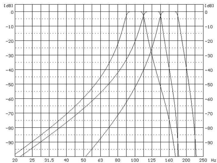
**1/3 octave filters for 125 Hz 1/1 octave filter**
