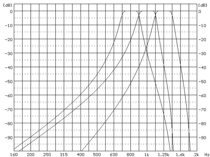
**1/3 octave filters for 1.00 kHz 1/1 octave filter**
