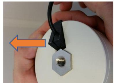
2. Release the cable from the seal.
