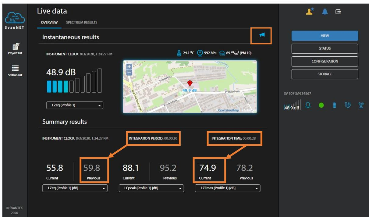
The map field is used to show the instrument's position and meteorological data.
