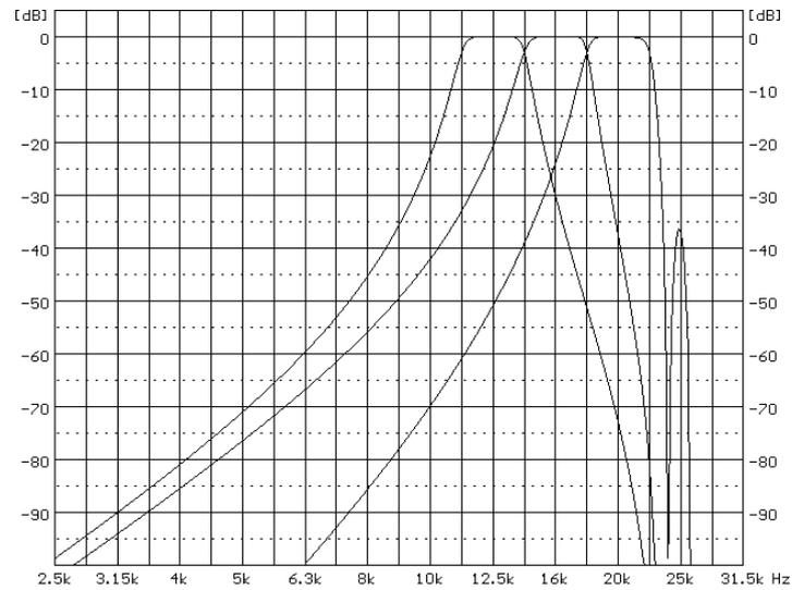
**1/3 octave filters for 16.0 kHz 1/1 octave filter**
