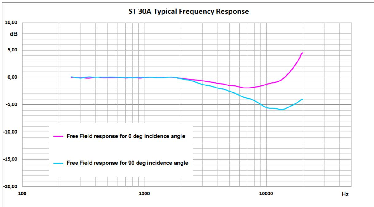
**Table C.1.4.** ST 30A typical Free Field response for 0 deg and 90 deg incidence angle
