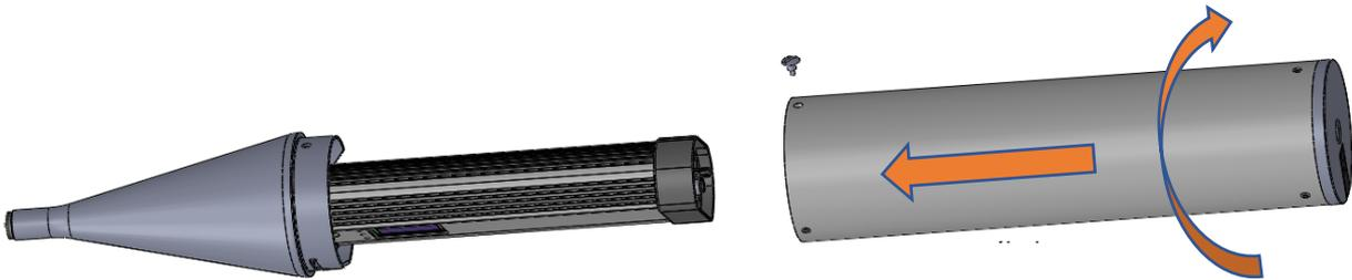
12. Pull the cable out of the lower casing.
