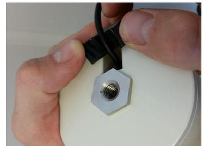
3. Unscrew in the fixing bolt in the upper part of the lower casing.
