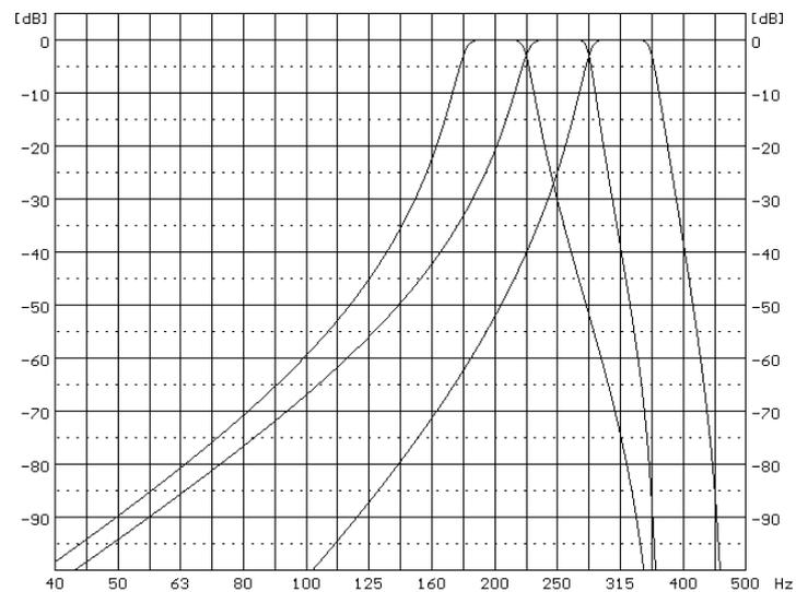
**1/3 octave filters for 250 Hz 1/1 octave filter**
