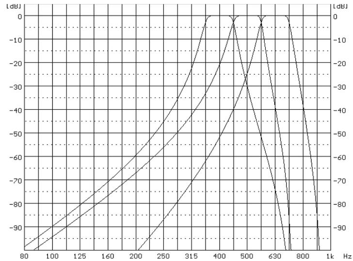
**1/3 octave filters for 500 Hz 1/1 octave filter**
