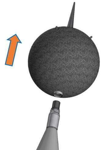
4. Attach the acoustic calibrator (SV 36 or equivalent 114 dB/1000 Hz) carefully on the microphone.
