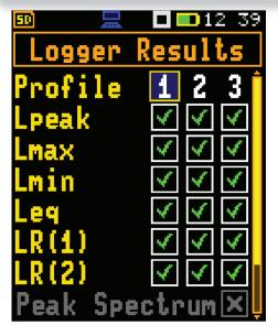
The SV 307 is capable of logging summary results (SR) and spectral data with interval steps down to 1 second. Also time history results (TH) down to 100 milliseconds.
