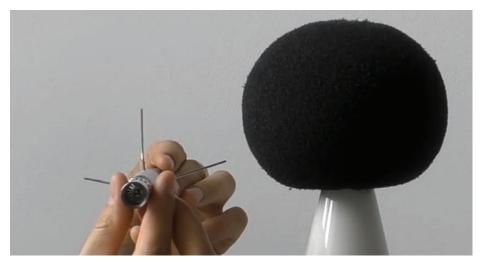
The ASC is based on a small speaker and the three MEMS microphones in the SV 307. Activation of the ASC enables the speaker and triggers an alarm if any of the three MEMS microphones reports a different noise level than the others.
