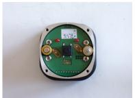
c) take off the cover and remove discharged batteries
