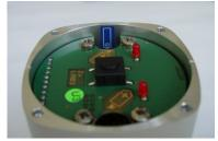
e) put on the cover so that the diodes fit the corresponding holes in it
