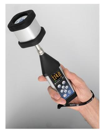
Picture 2. Calibration of the SVAN 971 sound level meter with a 1/2" measurement microphone
