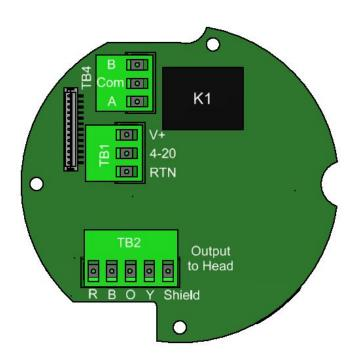
Figure 6 - 700-0102-01 3-Wire Power Supply
