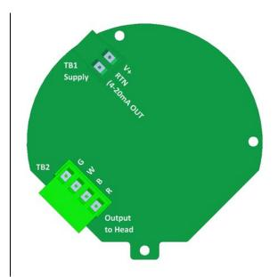
Figure 4 - 700-0100-01 2-Wire Power Supply
