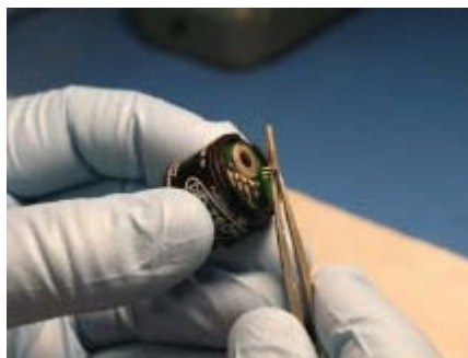
Figure 7–12. Installing the Cell Assembly
