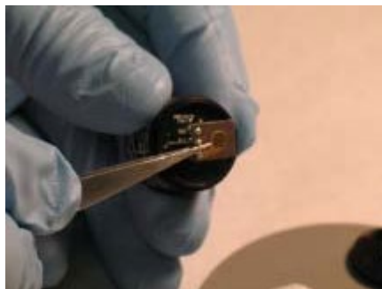
Figure 7-7. Removing the Cell Assembly
