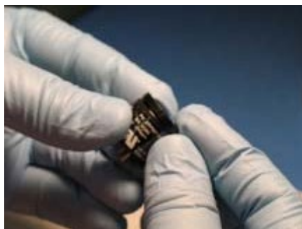
Figure 7-15. Aligning the Cap Key
