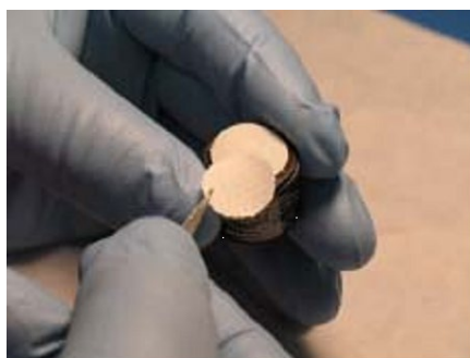
Figure 7-14. Placing the Filter Media
