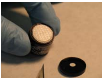
Figure 7-5. Removing the Filter Media
