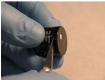
Figure 7-4. Removing the Filter Cap
