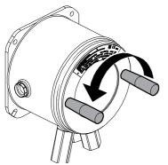
Turn counter-clockwise to unscrew the front cover.
