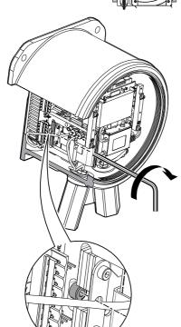
If the module is in its correct position, the screws will engage in the threads and turn freely.
