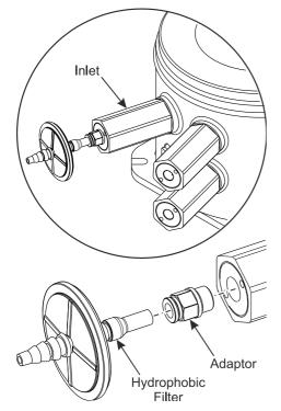
Ensure the external hydrophobic filter and any exhaust or inlet probe lines are connected.
