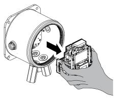
When the captive screws are completely loose, grip the sides of the frame of the Detection Module, as shown, to remove it from the Housing Module.
