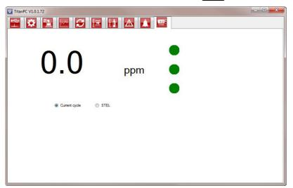
This tab displays in real time what is displayed on the Titan screen. A radio button allows the user to switch between the current cycle reading and the calculated STEL.
