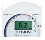
LEDs Green Titan is operating correctly.
