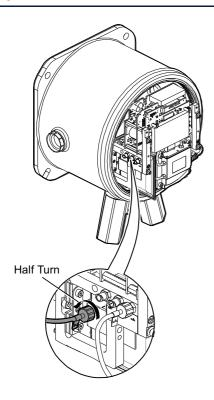
Ensure the pneumatic tubes are properly identified for later connection to the correct connectors.
