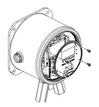
Use a 2mm allen-key to remove the four faceplate screws.
