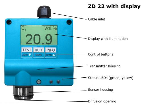
The gas sensor and the transmitter electronics are installed in the transmitter housing. The electronics convert the measurement signal into a gas concentration and indicates it with an analog current signal of 4-20mA or 0.2-1mA or with a digital RS485 bus signal in the MODBUS RTU protocol. The gas concentration and status information are displayed on the display version.
