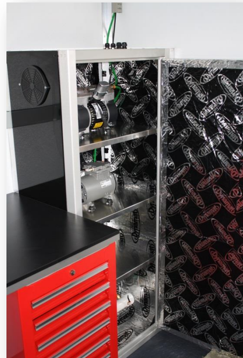
Workbench, Tool Chest, and Pump Cabinet to reduce heat, noise, and vibration
