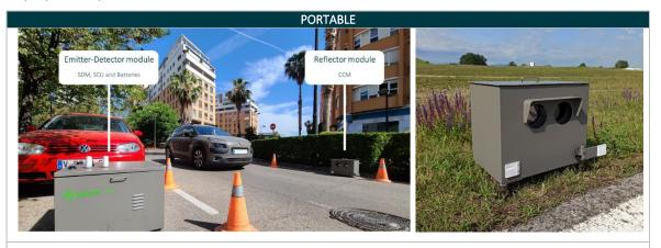
The RSD6000 can be quickly deployed on the roadside in protective boxes, for quick and easy deployment. This configuration allows the RSD6000 to be easily transported and placed at a specific site without any prior preparation.
