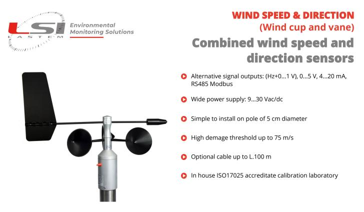
Combined wind speed and wind direction sensor. This sensor range includes, in a single apparatus, transducers for both wind speed and wind direction measurement. Its use simplifies installation requirements, other than being smaller, lighter and cheaper than the general 2-sensors kit. Accuracy and thresholds are anyway near to be comparable with 2-sensors cup and vane kit alternatives. Different data output signals are available.
