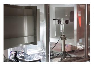
▶ LSI LASTEM is an ISO17025 accreditated laboratory for air speed measurements. All sensors manufactured are tested inside this laboratory. LSI LASTEM provides Test report for any sensor supplied and on request, ISO17025 or ISO9001 calibration certificates (see Accessories list).
