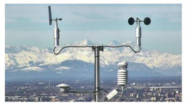
S Wind speed sensor can be mounted together with wind direction sensor using the DYA046 coupling bar. On the same coupling bar room for additional sensor as Temperature&RH% and Radiation sensors is available.
