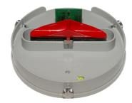
The LSI LASTEM's rain gauges has been developed taking the Class A standard as a reference (UNI EN 17277:2020 (Hydrometry - Measurement requirements and classification of rainfall intensity measuring instruments). The Class A assures an accuracy over intensity of 3% within 0...300 mm/hr range.
