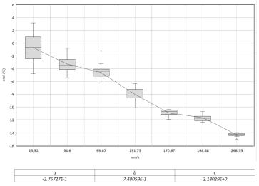
• Curve of relative percentage errors as a function of intensity, obtained following the calibration procedure. It is possible to interpolate the curve with a power function and obtain the parameters a, b and c for the correction of the rainfall intensity data measured by the rain gauge. Each rain gauge needs its own calibration to be classified as Class A.
