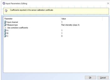
• Alpha-Log and Pluvi-ONE data loggers have the corrective formula for precipitation intensities on board. Following the calibration procedure, parameters a, b and c are obtained to be inserted in the 3DOM configuration software. Thanks to this setting the values recorded by the data logger are already correct and have a relative residual error <± 3% (Class A).
