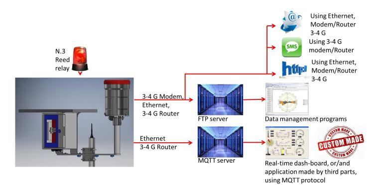
In the picture above there is a general overview of the Alpha-Log data logger data communication/management possibilities. Communication ports/device and data format (Ethernet, RS232-485 ports. HTTP, FTP MQTT protocols), power outputs and alarms by SMS are available in a single device.
