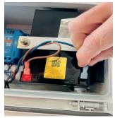
4- During commissioning, reconnect the disconnected terminal (blue or black wire) to the negative (-) terminal of the battery.
