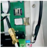
2- Insert the SIM card, making sure it is properly oriented with the notch on the left.
