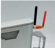
4- Stand the device upright and deploy the communication antennas as shown in the picture, then tighten them (they are folded and loose when delivered).
