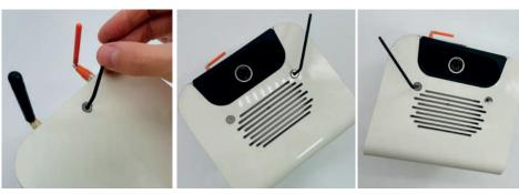
1- Remove the screw located on the top of the device using the 2.5 mm Allen key
