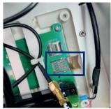
1- Locate the SIM card slot, then slide the top latch to the right to open it.
